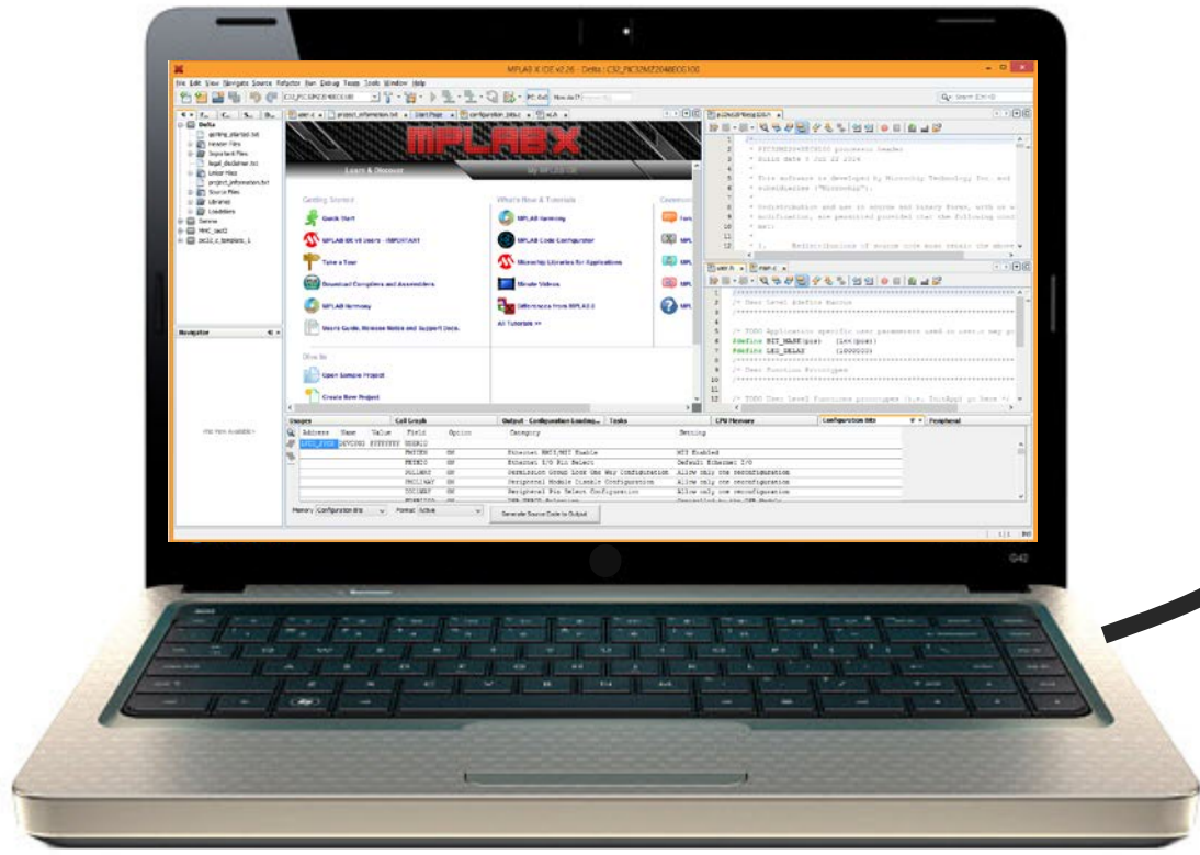
MPLAB X IDE on Development PC Create and debug programs in C, C++, assembly language here with Microchip's professional tool suite.
